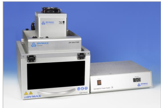
Dymax 5000 UV-Curing Flood-Lamp System Shown with Light Shield protective enclosure and ZIP™ shutter. Ideal for single component or batch curing processes requiring moderate intensity and a 5" x 5" (12.7 cm x 12.7 cm) cure area. CE Marked ECE Series Flood Systems available for European production facilities.
