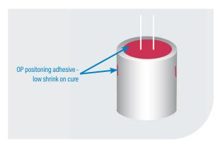
Positioning Laser Diodes (VCSEL's)
