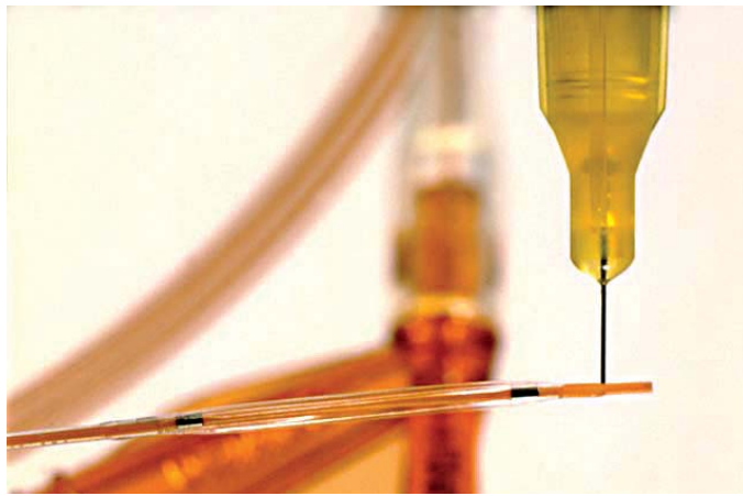
Adhesives are used to join tubing to catheters. Photo courtesy Dymax Corp.
