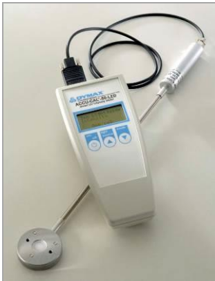
Figure 4. Attach Detector to Radiometer
