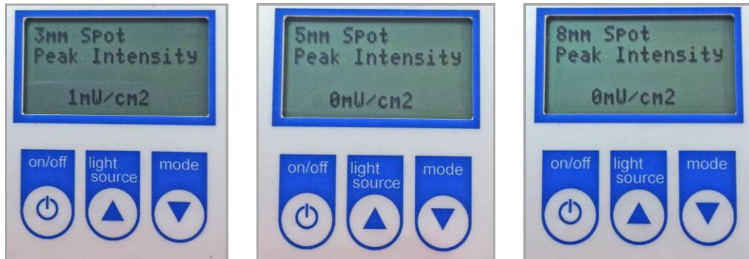
Figure 13. Spot Mode Screens (Shown in Peak Intensity Mode)
