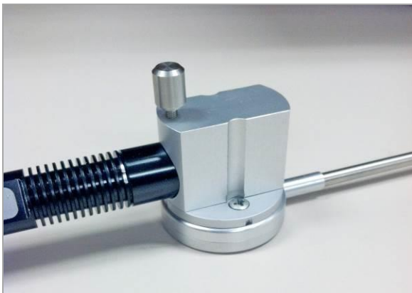
Figure 12. Insert LED Wand into Optical Adapter
