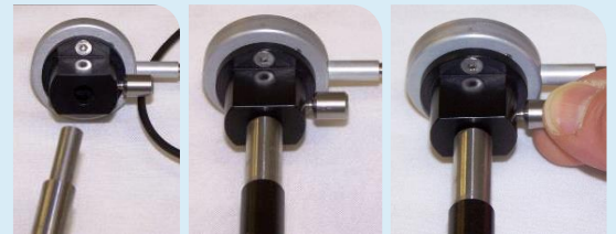
Figure 8. Attach Lightguide Adapter to Lightguide (Step 4)
