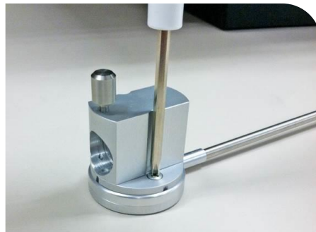
Figure 16. Attach Optic Adapter to Detector
