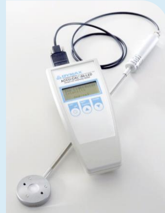
Figure 6. Attach Detector to Radiometer
