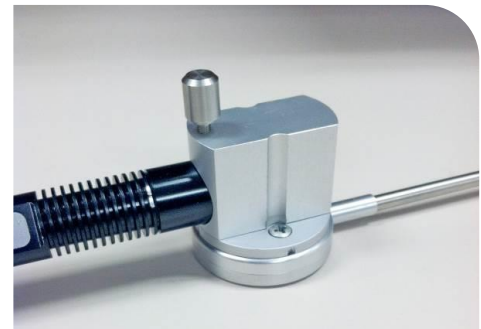
Figure 17. Insert LED Head into Optical Adapter
