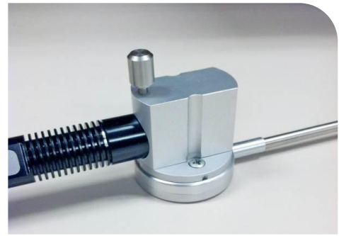
Figure 17. Insert LED Head into Optical Adapter
