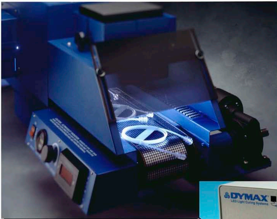
Top photo: Semiautomated conveyor curing of tube sets. Bottom photo: Manual LED curing of adhesives for bonding connectors and tubing.
