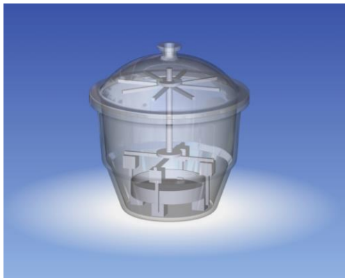
Figure 5. Representation of a flowers of sulfur test chamber
