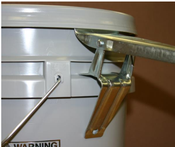
Figure 3. Place the Pail Tool Hook under the Cover Skirt and Push Downward on the Pail Tool Handle
