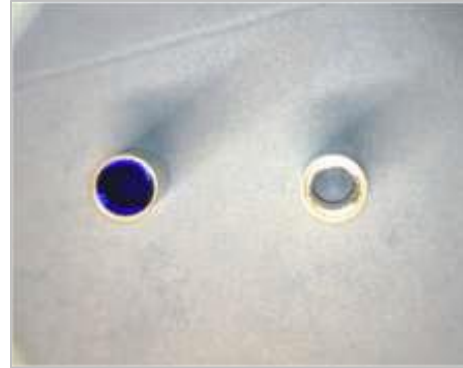
Figure 6. End-of-Wand Heat-Reducing Filter (Left) & Lightguide End Protector (Right)
