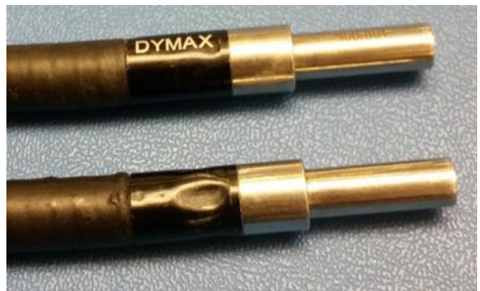
Figure 8. Damaged Lightguide Caused by Over Tightening
