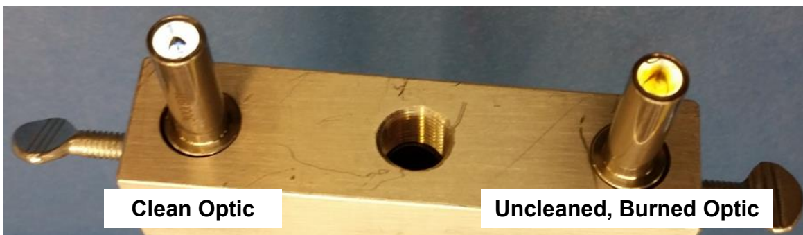
Figure 4. Damaged, Burned Lens
