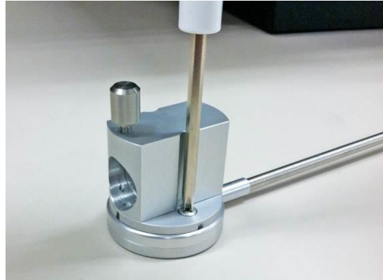
Figure 11. Attach Optic Adapter to Detector
