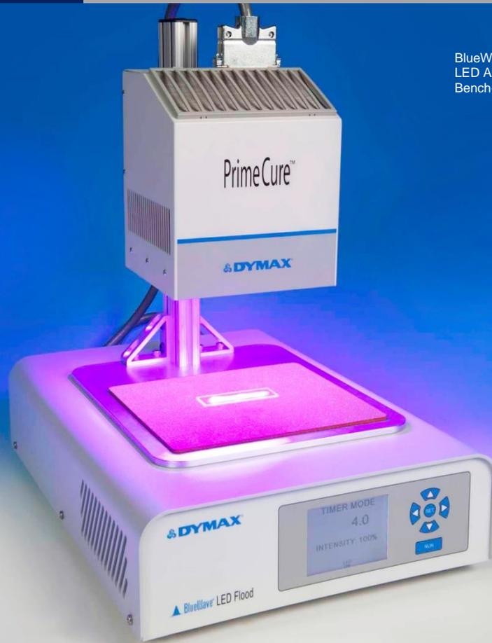
BlueWave<sup>®</sup> LED Flood with PrimeCure<sup>™</sup> LED Array and Standard Mounting Stand in Bench-Top Configuration
