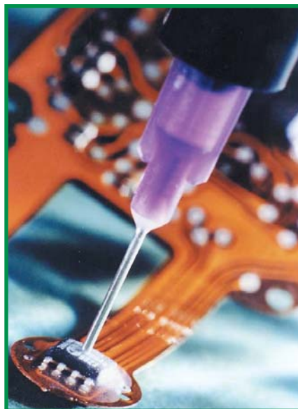
FIGURE 5: A number of UV coatings and encapsulants are available for bonding to difficult substrates such as Kapton and Mylar. Other adhesion problems may be encountered when coating over certain solder masks.
