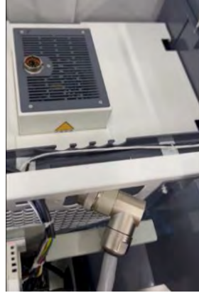
Figure 24. Cable Connector goes through the Wire Slot
