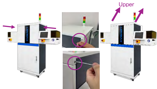
Figure 16. Open the Upper Cover
