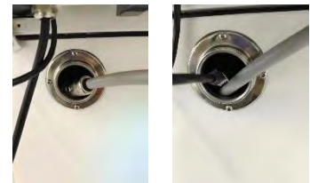
Install Connector and Network Wire on the Controller Connection
