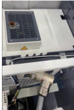
Figure 24. Cable Connector goes through the Wire Slot
