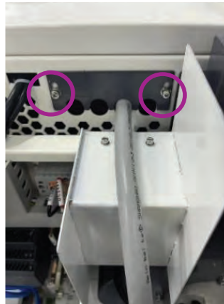
Figure 26. Install the Wire Pressing Plate, and add the Screws
