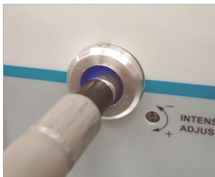
Figure 6. Insert Lightguide into Lightguide Mount
