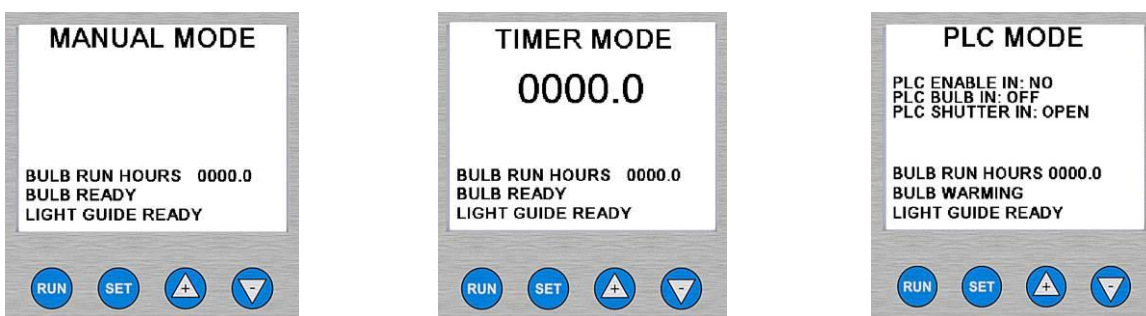
Figure 12. Mode Start-up Screens (Left to Right: Manual Mode, Timer Mode, PLC Mode)
