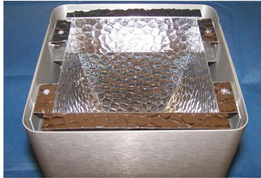
3. Place the Mounting Plate onto the Reflector Housing (Figure 6) and then place the Air Plenum on top of the Mounting Plate (Figure 7). Attach all three components together with four new M4 x 25 mm screws.
