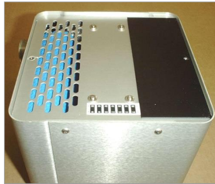
Figure 12. Temperature Control Plate and Temperature Indicating Strip, Installed
