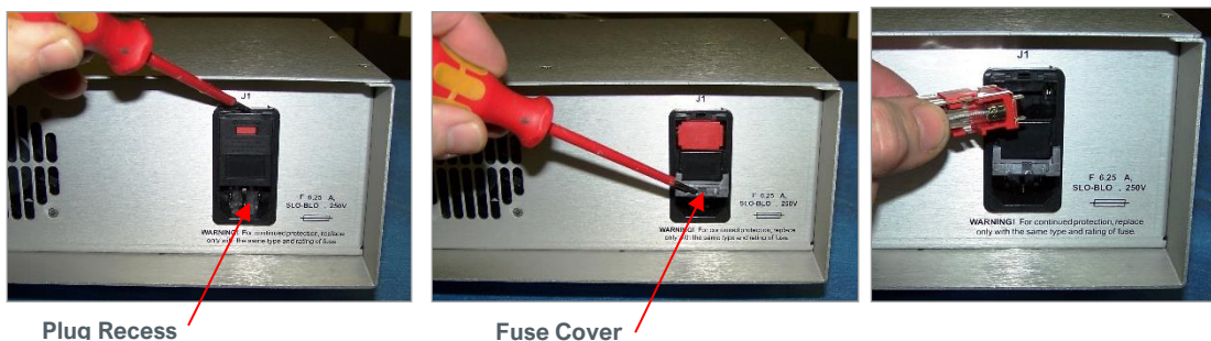
Figure 16. Replacing Fuses in the Power Supply
