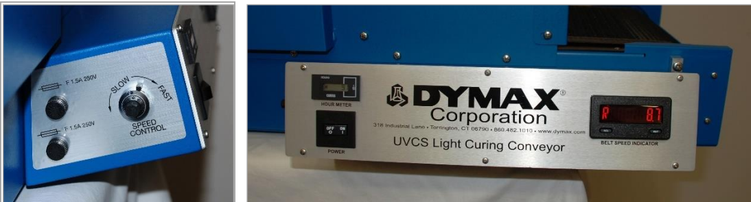
Figure 6. Conveyor Control Panel
