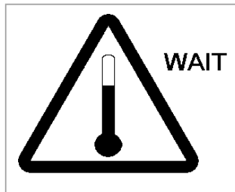
Figure 29. LED Head Has Overheated
