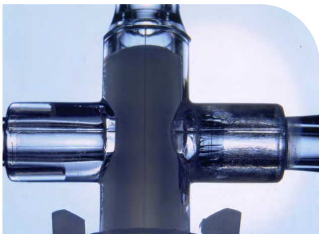
Figure 1. Stress Cracking on Plastic Tube Set
