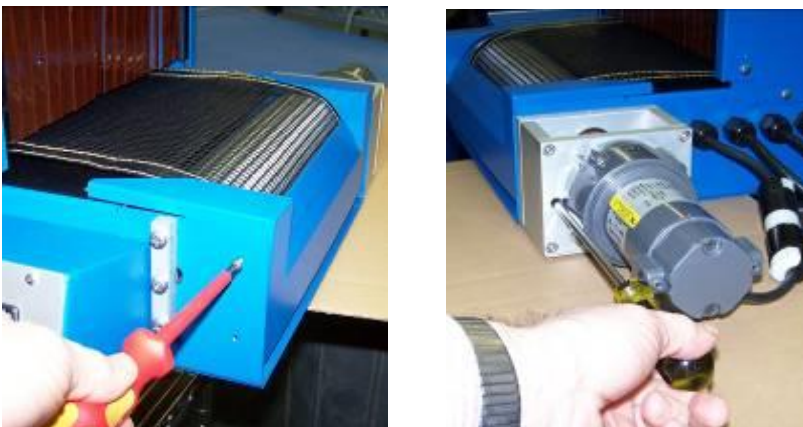
Figure 22. Installing Pinch Guard (front & back)
