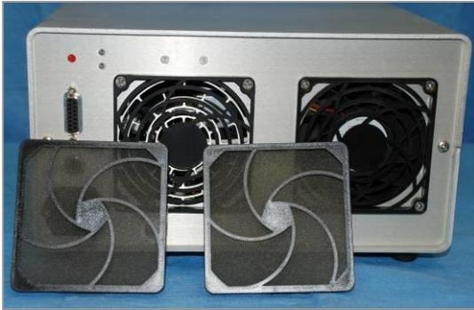
Figure 28. Exhaust Fans with Fan Filters Removed
