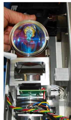
Figure 14. Remove Bulb from Bulb Mount
