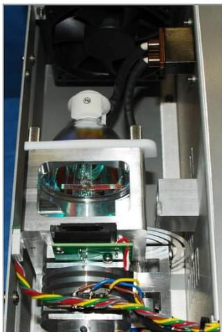
Figure 12. Bulb Installed in Bulb Mount
