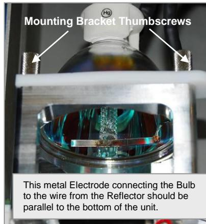
Figure 21. Bulb Electrode
