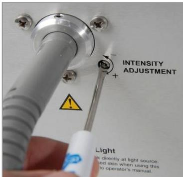
**Figure 7.** Intensity Adjustment with Tool
