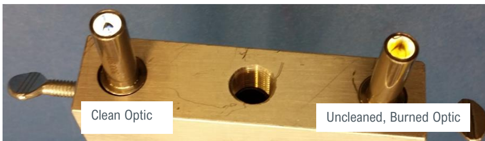
Figure 4. Damaged, Burned Lens
