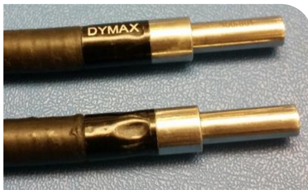
Figure 8. Damaged Lightguide Caused by Over Tightening
