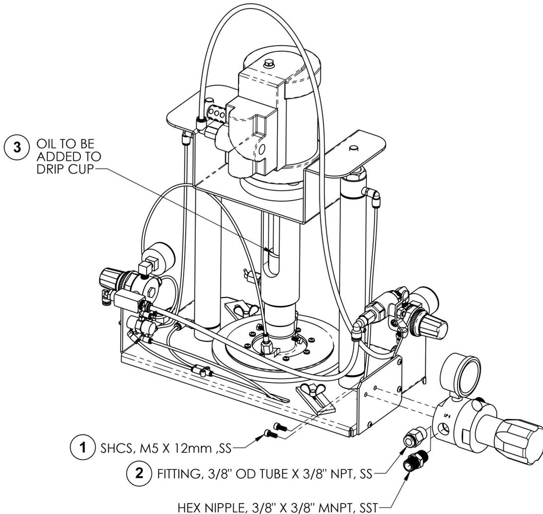
1. Mount the regulator to the plate on the ramp pump using the supplied 2 socket head cap screws (SHCS). Do not exceed 25 ft/lbs.
