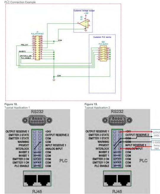
**Note:** The Input/Output terminal block is included in the packaging, with the jumper wires inserted. When the terminal block is installed, the controller will enter PLC mode. PLC mode disables commands and parameter settings from the HMI. To set parameters from the HMI, the terminal block must be removed, or the connection between the PLC Enable and COM pins (1 and 2) must be disconnected.
