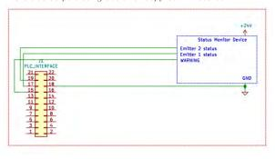
**Figure 22.** Examples of Customer Configurations for Monitoring Outputs
