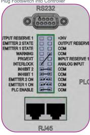
Note: The Input/Output terminal block is included in the packaging, with the jumper wires inserted. When the terminal block is installed, the controller will enter PLC mode. PLC mode disables commands and parameter setting from the HMI. To set parameters from the HMI, the terminal block must be removed, or the connection between the PLC Enable and COM pins (1 and 2) must
