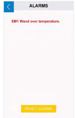
Figure 38. Temperature Alarm Screen
