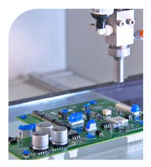
atomized or non-atomized technique. Atomized techniques introduce air to the material and produce a fine mist or spray. This method is the most common for conformal coating. Spray pattern widths can vary from 3.18 mm [0.125 in] to over 50 mm [2 in]. A thickness of 200 microns [0.008 in] or greater may be achieved in a single pass. Applied coating thickness and width are functions of the robot speed, air pressure, height off the work surface, and flow control on the applicator.
