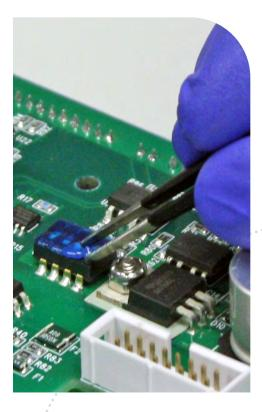
**Best Practice:** Clean boards prior to applying conformal coatings in order to eliminate contaminants and maximize wetting and adhesion.
