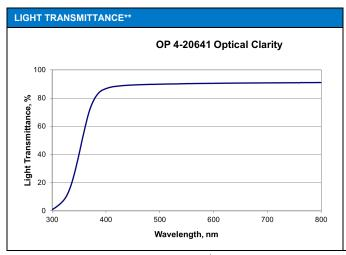
\*\* Measured at 0.03 mm [0.001" in] per DSTM-501<sup>‡</sup>
