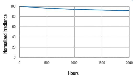
Figure 6. LED Degradion Testing - PrimeCure®
