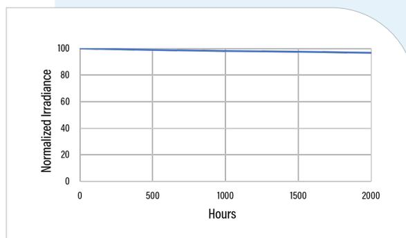
Figure 7. LED Degradion Testing - VisiCure®
