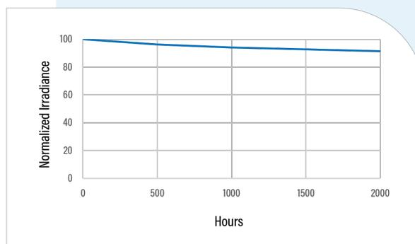
Figure 6. LED Degradion Testing - PrimeCure®
