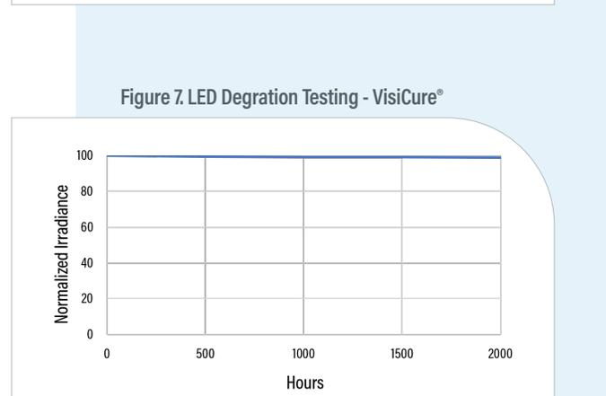
Note: Testing conducted at 70°F +/-3°F and 30% +/-10% Relative Humidity
