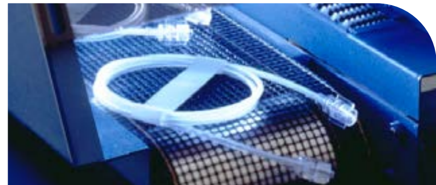
Tube Sets Traveling Through Light-Curing Conveyor System
