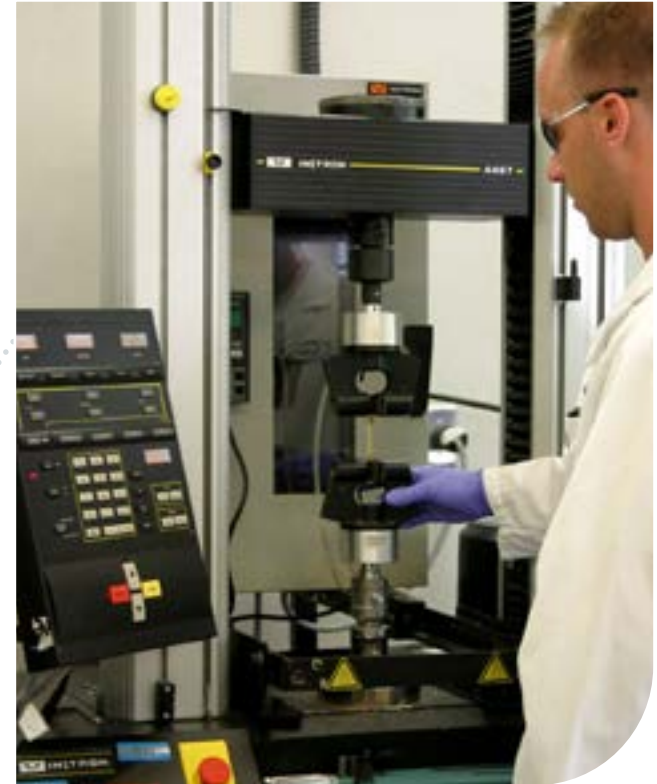
Adhesive Being Tested for Strength
