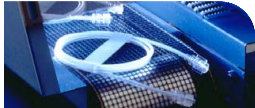
Tube Sets Traveling Through Light-Curing Conveyor System
