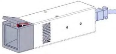
4. Slide the damaged glass cover out (Figure 6), taking care not to touch the metallic reflector surfaces.
