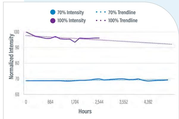
Figure 9. LED Degradation Testing - VisiCure
