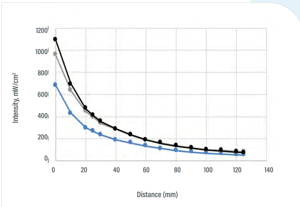
Figure 5. Intensities at Various Working Distances
