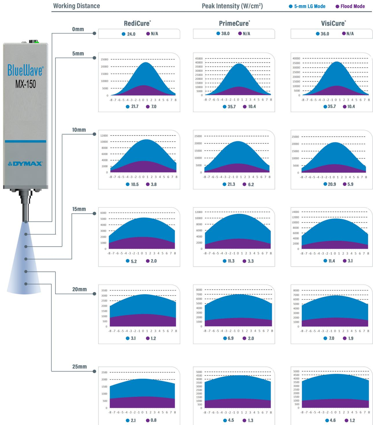
\* Dymax recommends using the 5-mm lightguide source mode on the ACCU-CAL™ 50-LED, when measuring at 0 mm with the provided adapter in the ACCU-CAL kit. If measurements are made at greater working distance, Dymax recommends using the flood mode source for measurements. For convenience, both numbers are provided in this chart.
