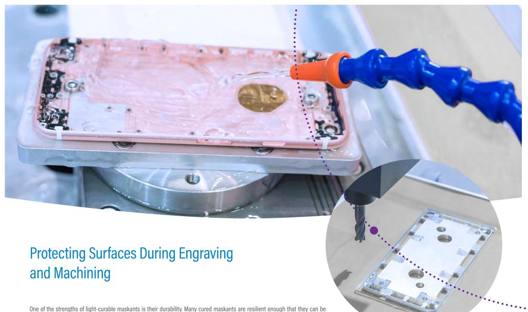
machined through, without the remaining mask lifting and compromising protection. They can also withstand various watersoluble and oil-based coolants used in machining. This creates clean, crisp edges and can be beneficial when engraving logos, safety warning, or other items on parts or when machining out areas for buttons, speaker areas, and other jacks.
