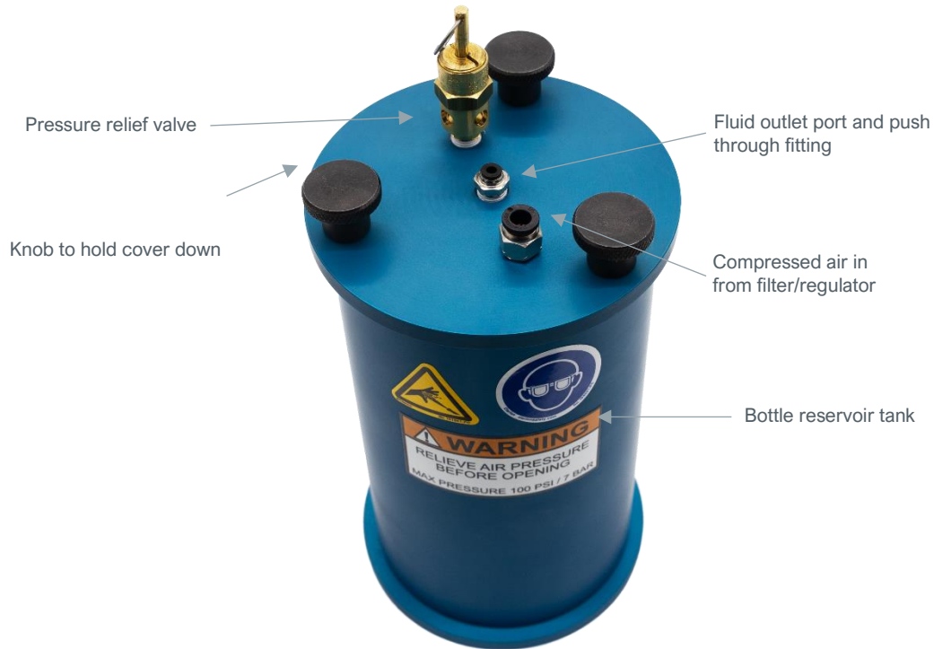
Figure 1. Pressure Pot Components
