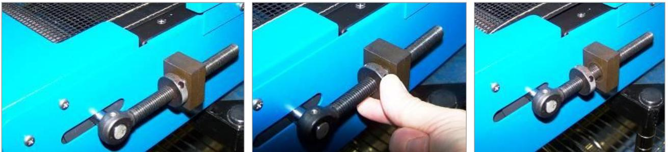
3. Manually move the belt splice to the end of the conveyor. Remove the fiberglass rod that ties the ends of the belt together. Remove the belt.
