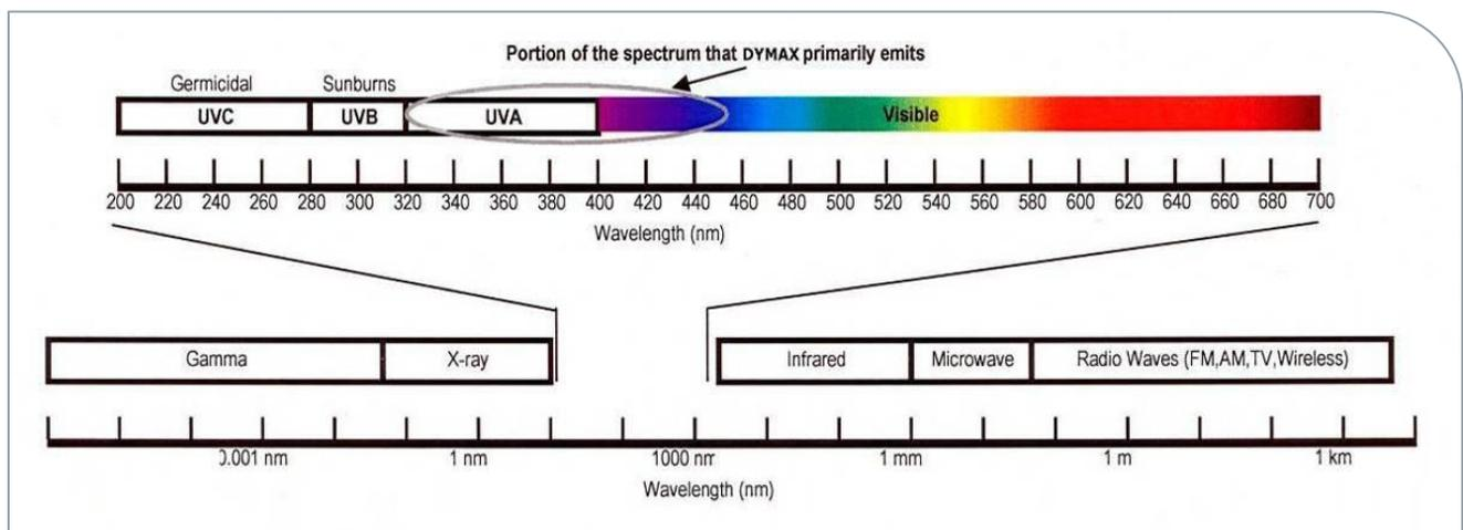
The human eye cannot detect “pure” UV light, only visible light. A radiometer should be used to measure stray UV light to confirm the safety of a UV light-curing process. A workstation that exposes an operator to more than 1 mW/cm<sup>2</sup> of UVA continuously should be redesigned.
