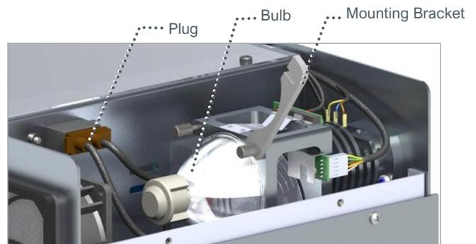
5. Unpack the new Bulb. Take care not to bend the flat Electrode in the Bulb (Figure 42).
