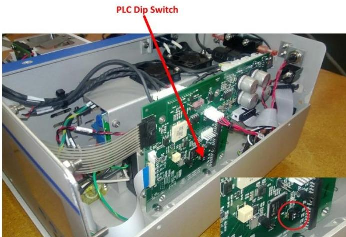
4. Adjust the PLC Switch (see below) and replace the Inner and Outer Covers.
