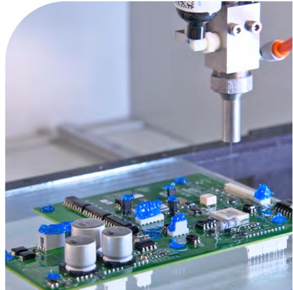
introduce air to the material and produce a fine mist or spray. This method is the most common for conformal coating. Spray pattern widths can vary from 3.18 mm [0.125 in] to over 50 mm [2 in]. A thickness of 200 microns [0.008 in] or greater may be achieved in a single pass. Applied coating thickness and width are functions of the robot speed, air pressure, height off the work surface, and flow control on the applicator.
