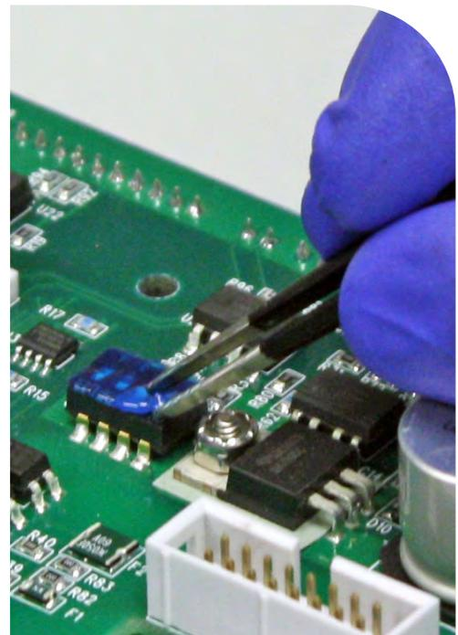
**Best Practice:** Clean boards prior to applying conformal coatings in order to eliminate contaminants and maximize wetting and adhesion.
