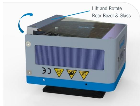
3. Remove the foam rubber seals from the grooves in the bezels. Remove the release liner from the pressure-sensitive tape on the replacement foam seals and install/adhere to the grooves in the front and rear bezels (Figure 3).
