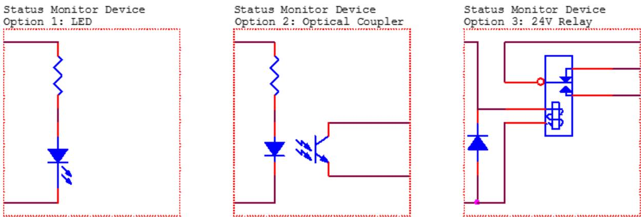
PLC Power channel is a 24V source available for use to drive PLC logic but must be current limited using pull-down resistors to protect the BlueWave AX-550 V2.0 when directly attached to the I/O channels through the PLC connector.
