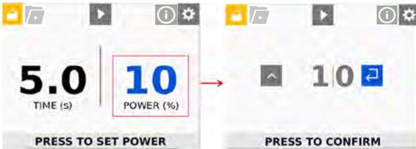
**Note:** the minimum power value to configure LED intensity must be 10% to avoid linearity in irradiation area intensity. If the set value is less than 10, it will be taken as an invalid setting and it will be necessary to enter a new value.
