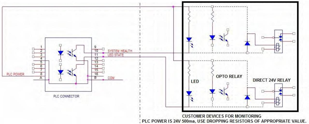
PLC Power channel is a 24V source available for use to drive PLC logic but must be current limited using pull-down resistors to protect the BlueWave AX-550 V2.0 when directly attached to the I/O channels through the PLC connector.
