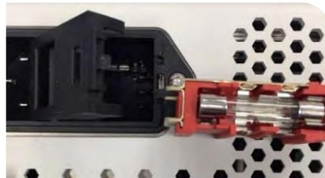
5. Verify the installation is correct by noting the word "FUSED" in the window of the fuse mount.
