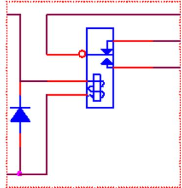
PLC Power channel is a 24V source available for use to drive PLC logic but must be current limited using pull-down resistors to protect the BlueWave AX-550 V2.0 when directly attached to the I/O channels through the PLC connector.
