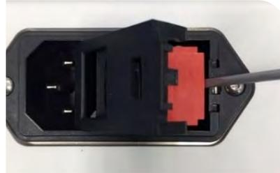
3. Take out the Fuse Holder. (Figure 51). *Note that the fuse holder is labeled for correct orientation.*
