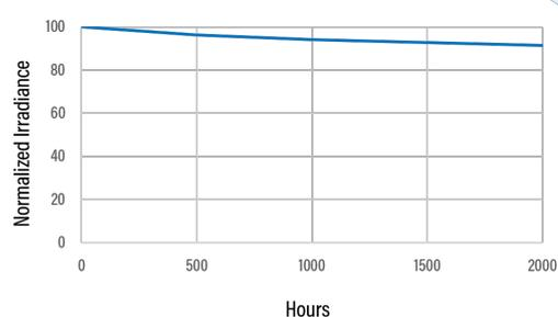
Figure 6. LED Degradion Testing - PrimeCure®
