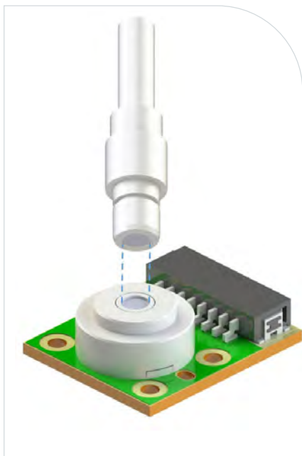
Figure 10. Aperture with 5-mm Lightguide
