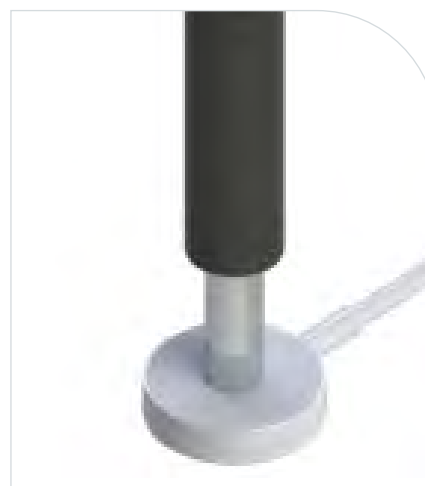
Figure 8. BlueWave® LED Prime Using a 8-mm Lightguide, Measured Directly on the Surface of the Radiometer
