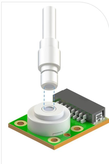
Figure 11. Aperture with 3-mm Lightguide
