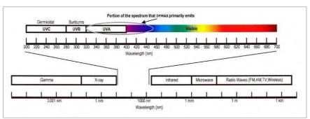
Standard Dymax light-curing systems have been designed primarily to emit UVA and Visible energy above 400 nm (Figure 1).
