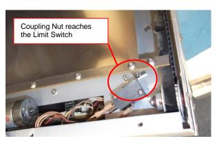
Figure 12. Rear Limit Switch
