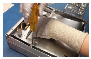
Figure 11. Tighten the M4 x 6 mm End Screws
