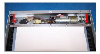
Figure 7. Loosen End Screws
