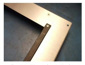
Figure 16. Install M3 x 6 mm Screws into Wear Strip
