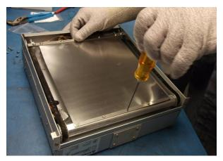
Figure 9. Install Curtain to Roller Bar with Five Retaining Screws
